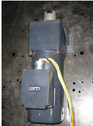
Figure 3-39 Induction motor for yaw brake
