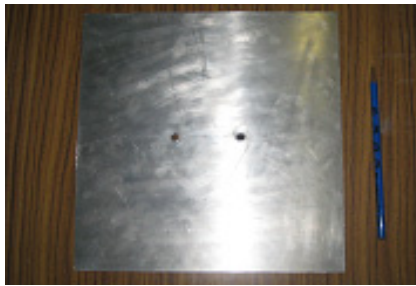
Figure 3-50 Tested tail fin 1 for restoring moment measurement
