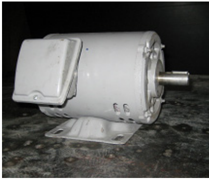
Figure 3-37 Induction motor for rotating rotor
