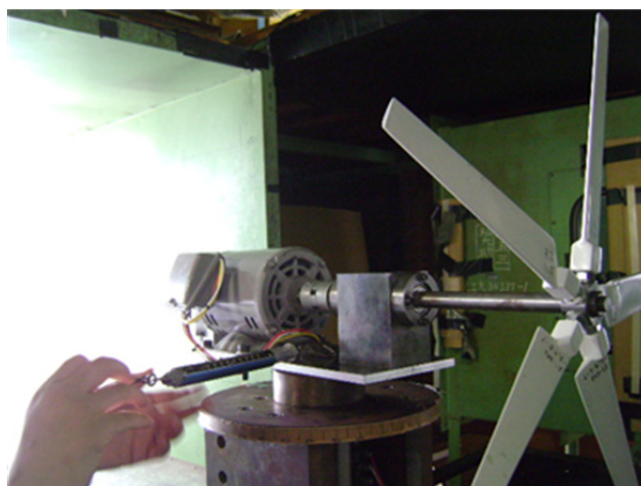
Figure 3-57 Measurement of slip ring static friction by spring scale
