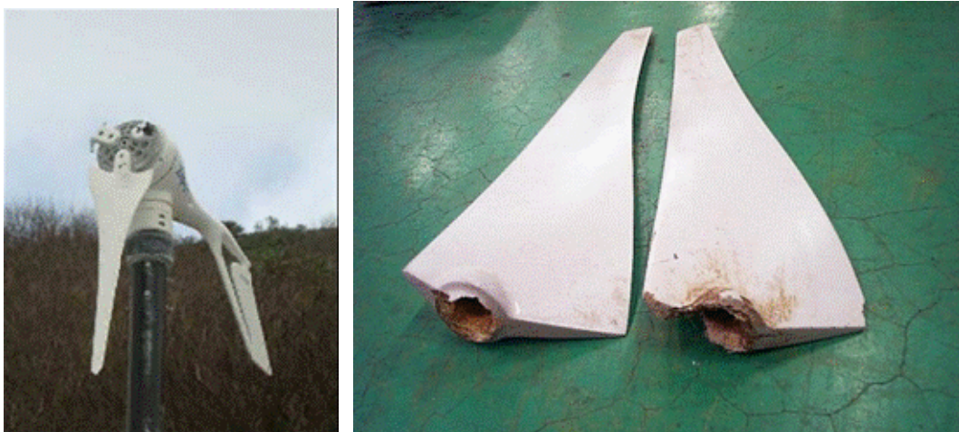
Figure 1-13 Damaged small wind turbine due to excessive moment in yawing [1-26]
