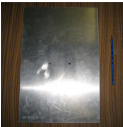
Figure 3-52 Tested tail fin 3 for restoring moment measurement
