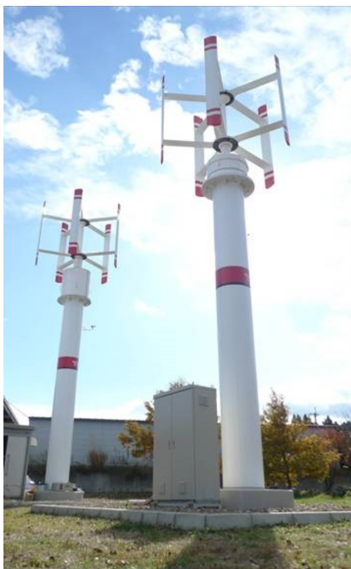
Fig.4.3 Vertical axis wind turbine generation system
