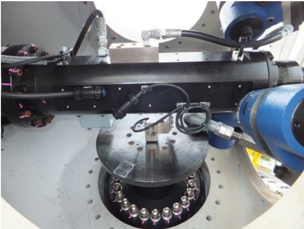
Fig.3.14 Internal structure of pitch actuator
