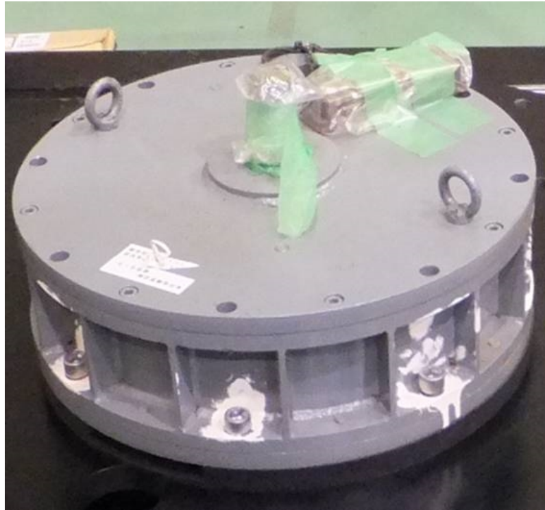
Fig.4.6 CC(Control Circuit) Less Generator
