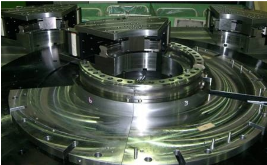
Fig.3.23 Assembling gearless Yaw driving system 1
