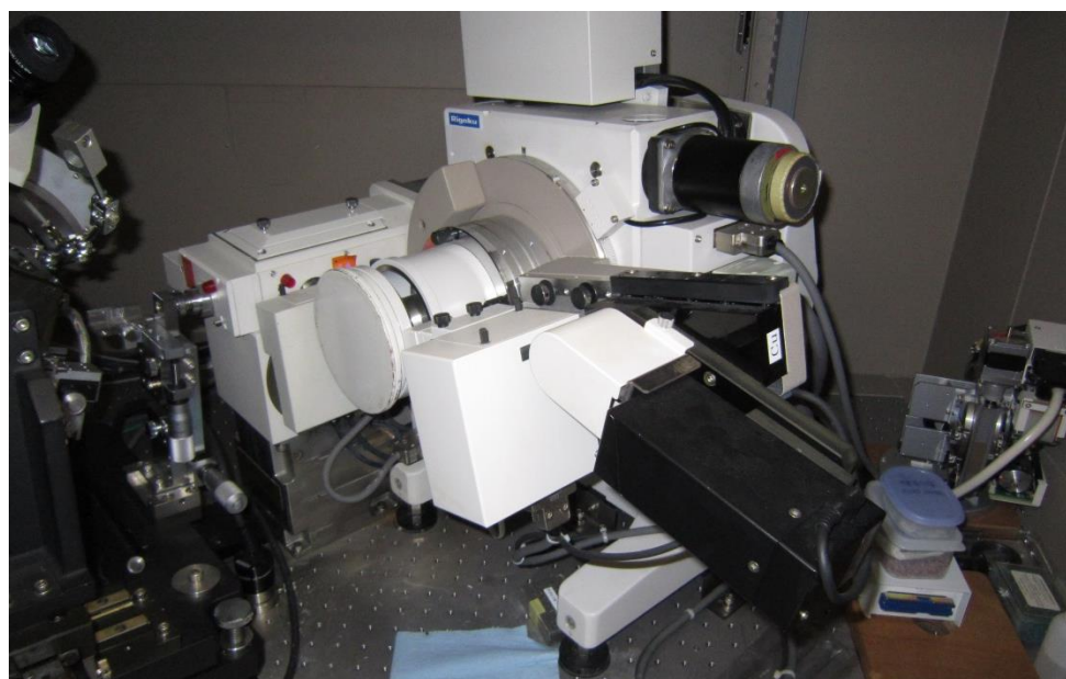
Fig. 5.2 X-ray diffractometer employed for evaluation of surface orientation distribution of the cold rolled SUS430 specimens.
