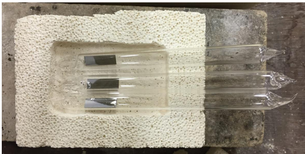
Fig. 5.1 The specimen enclosed in a SiO 2 glass tube with 8 mm in the internal diameter and 70 mm in the length in a vacuum of 10 Pa.
