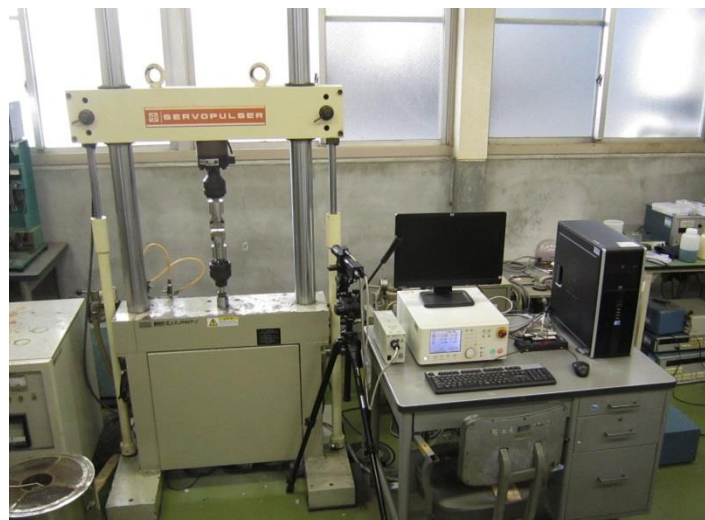
Fig. 3.6 Servo-hydraulic machine (Shimadzu Servopulser, EHF-EB2-10L) employed for high-cycle fatigue tests of SUS430 specimens.
