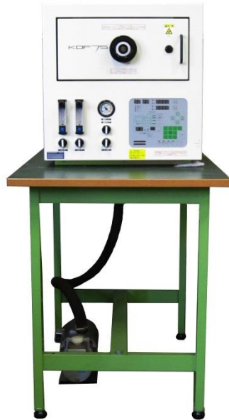
Fig. 3.2 Vacuum furnace (DENKEN, KDF-75 type) for solution treatment of SUS430 stainless steel sheet.
