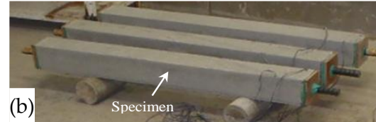
Fig. 2.5: (a) Apparatus for restraint stress test (b) Specimen stored in drying condition
