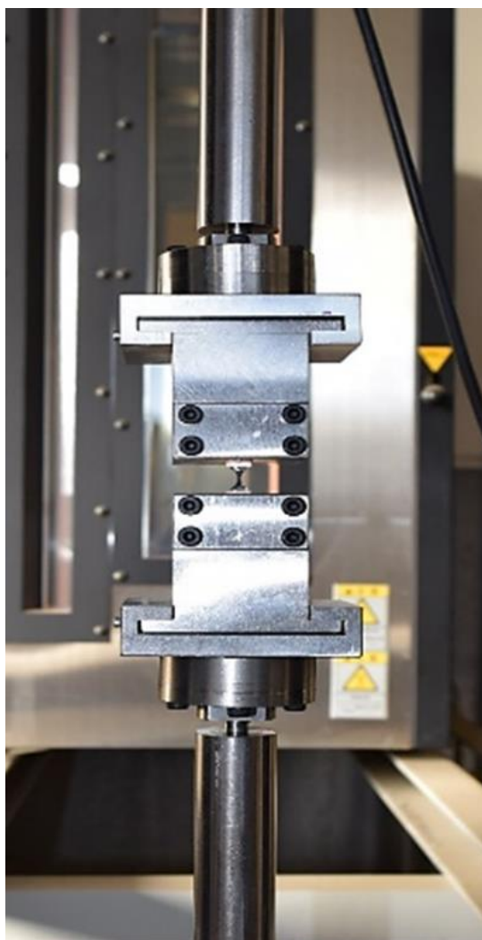
Fig. 4-3 Photo of a thin film specimen attached to a specially made chuck.
