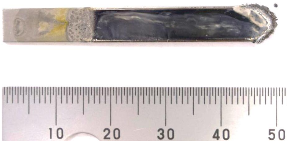
Fig. 3-2 Photo of multilayered nanocrystalline Fe-Ni specimen with 5 layers.
