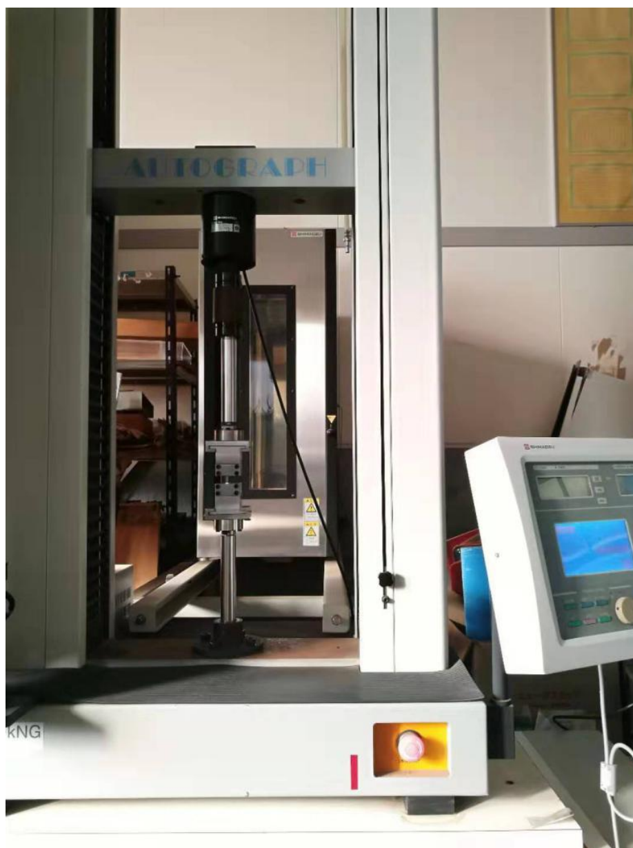
Fig. 4-4 Photo of tensile test machine (SHIMADZU AGS -10 kNG type).
