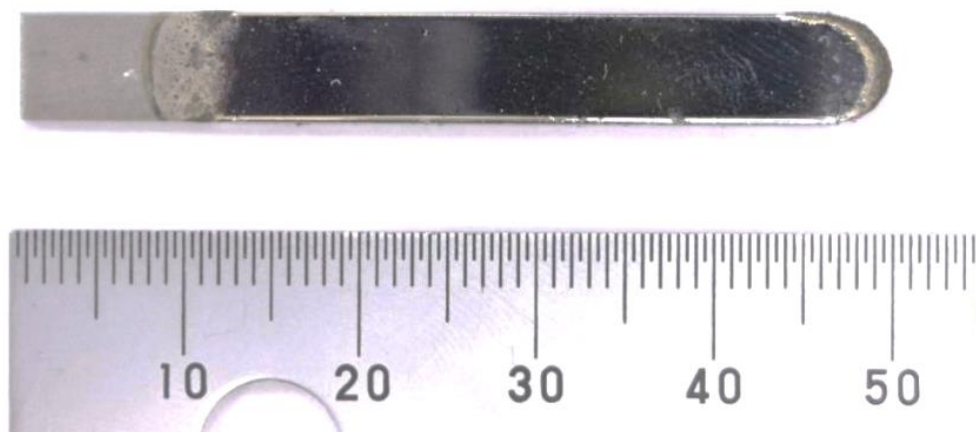
Fig. 2-2 Photo of electrodeposited nanocrystalline Fe-Ni specimen produced at 3.0 mA/mm 2 .
