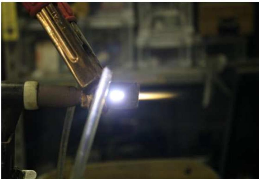
**Figure 3.4** Plasma jet generated by our thermal spray equipment
